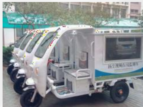
Vehicle dust monitoring on construction site
